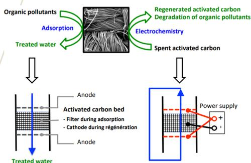
Water and wastewater treatment – Activated carbon regeneration
